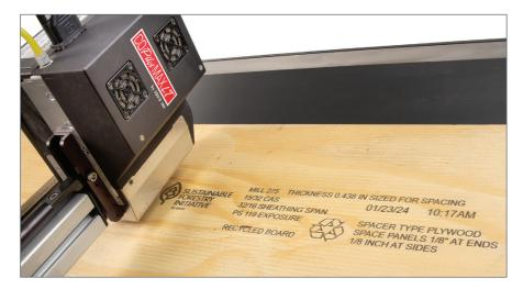
**1)** CoPilot Max LT allows reliable printing with an unprecedented 10-12mm throw distance.
